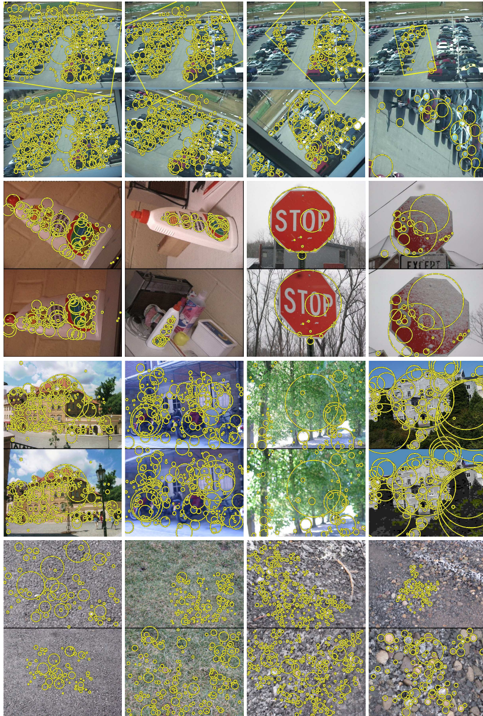
Fig. 6. Affine Ransac Image Matching Experiments. Row 1: four frames from a parking lot video sequence, showing affine alignment of bottom frame overlaid on top frame. The full video sequence of results is provided on our website. Row 2: left to right: shout3 to shout4; shout2 to was2 (images courtesy of Tinne Tuytelaars); stop sign; snowy stop sign. Row 3: kampa1 to kampa4 (images courtesy of Jiri Matas); bike1 to bike6; trees1 to trees5; ubc1 to ubc6. Row 4: natural textures: asphalt; grass; gravel; stones.
