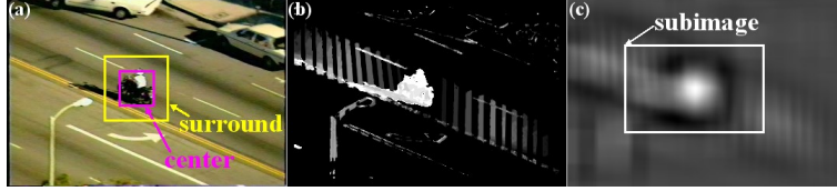
Figure 1: (a) Input image; (b) Motion detection by motion history images; (c) Mode and scale detection of the motion blob.
