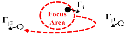
Figure 7. Focus Area. Kinematic constraints are less reliable across larger time windows. Because player motions are globally correlated, the affinity of two mid-level trajectories over large windows should agree with the overall movement trend of the focus area.
