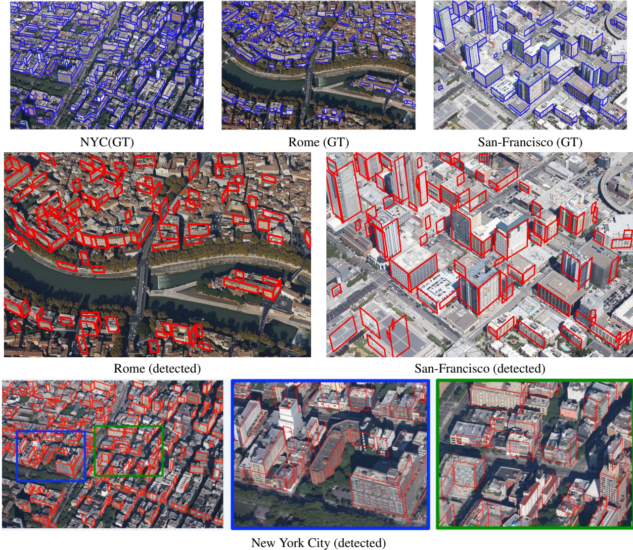
Figure 9. Top row: human labeled ground-truth facades (blue). Middle and bottom rows: facades detected (red) by our local-regularity driven algorithm.
