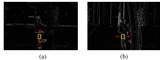
Fig.4. Adapting size of matching windows based on total horizontal (a) and vertical (b) gradients in the window.
