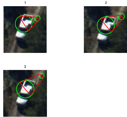
(a) Pair of unrelated parts. The circles indicate the scale and positions of the two parts; the corners of the quadrilaterals are the 4 points associated with each pair. These pair co-occurred only 3 times out of 20 but most unrelated pairs co-occurred for less than 3 times. Also notice how their pairwise geometry slowly departs from their initial one
