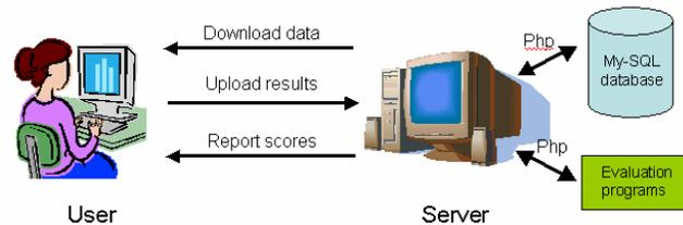
Figure 6. Framework for development of a tracking evaluation web page. PHP-enabled web scripts interface with a My-SQL database on a dedicated server, yielding great flexibility in designing and implementing web page functionality.
