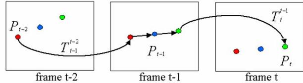
Figure 4: Prediction of current location of target,  $P_t$ , based on its previous two observed positions, and computed inter-frame displacements due to camera motion.
