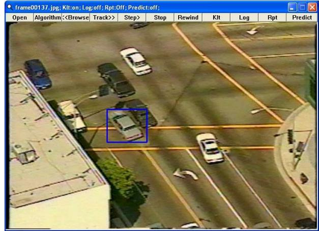
Figure 1: Screen capture of the real-time C tracking testbed, showing the tracked object bounding box and menu of interactive options displayed across the top of the graphical user interface.
