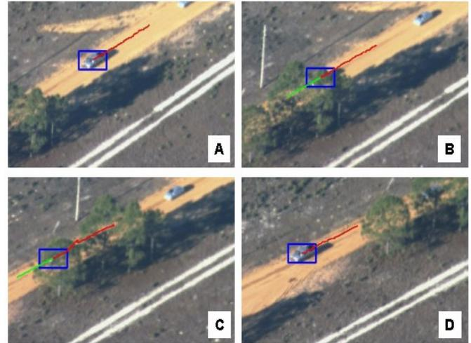
Figure 2. The testbed contains a motion prediction module that helps track objects through occlusion. The prediction method assumes object motion has constant velocity after compensating for affine motion of the scene background.
