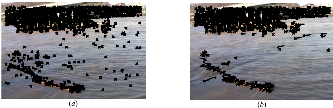
Figure 1 (a) The 1000 top features detected using a typical corner detector. Some but not many are detected on the water surface. (b) After tracking for one second at 10 frames per second most of the water features are lost whereas features on the land and a foreground object maintain track. While the camera has not moved, the water features have shifted considerably. In this example the detector and tracker used is that by [1] and it shows similar ability to exclude water surface features to our optical flow algorithm.
