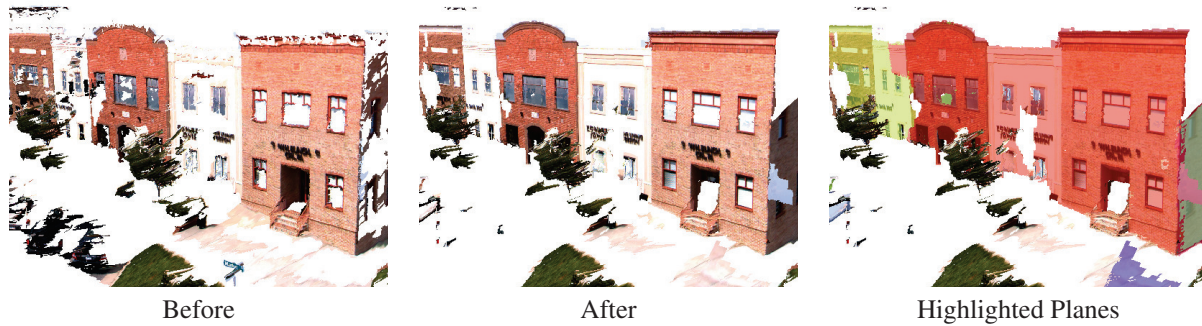
Figure 8. 3D model produced by our piecewise planar and non-planar stereo algorithm from 200 images (20 depthmaps).
