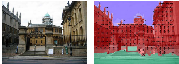
Figure 1: Geometric context from a single image: ground (green), sky (blue), vertical regions (red) subdivided into planar orientations (arrows) and non-planar solid ('x') and porous ('o').
