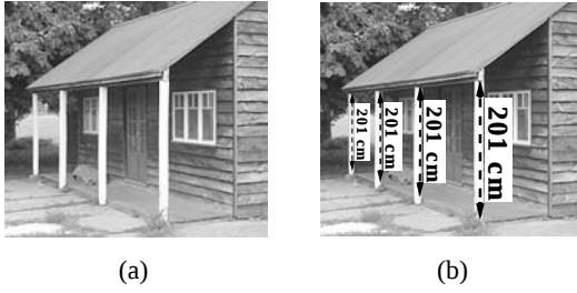
Figure 7: An example of measuring heights from a single image. (a) The four pillars have the same height in the world, although their images clearly are not of the same length due to perspective effects. (b) As shown, however, all pillars are correctly measured to have the same height.
